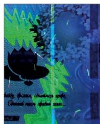
Under an ultra-violet light, portions of a polymer security thread, which is fully embedded in the paper, glow yellow and light blue.
