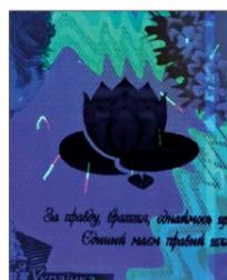
Under an ultra-violet light, security fibers that are scattered randomly in the paper and invisible in daylight, glow red and green.
